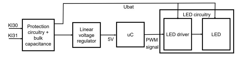
Pins KL30 - KL31 - input voltage. Nominal value U= 14 V. Range: U = 8...16 V. Average current consumption should be <100 mA in total taking into account that LED nominal DC current for required brightness is 80 mA. The LED brightness is proportional to average LED current. LED is driven by PWM signal with frequency 200 Hz. The PWM is used to do the brightness correction – LED brightness should keeps constant for the whole input voltage range.
