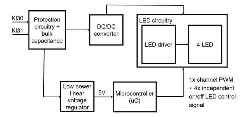
Pins KL30 - KL31 - input voltage. Nominal value U= 14 V. Range: U = 8...16 V. LEDs circuitry contains 4 independently controlled LED, each one consumes 20 mA of current. Common current consumption at KL30 should be <100 mA.
