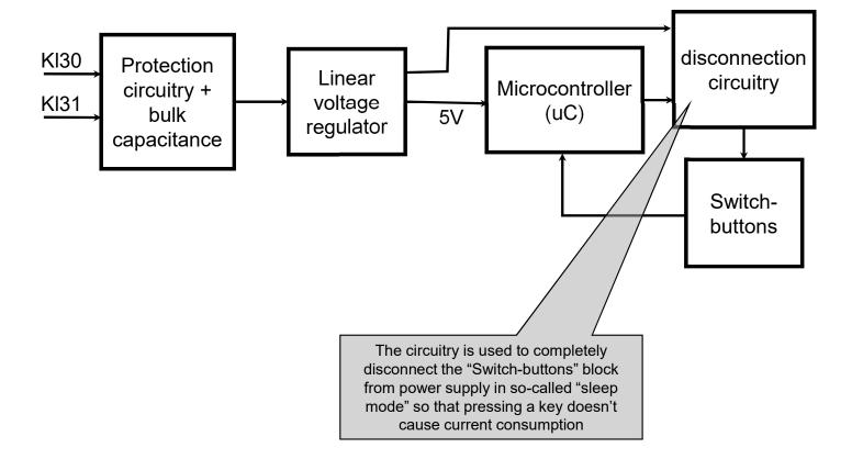
Pins KL30 - KL31 – input voltage.
